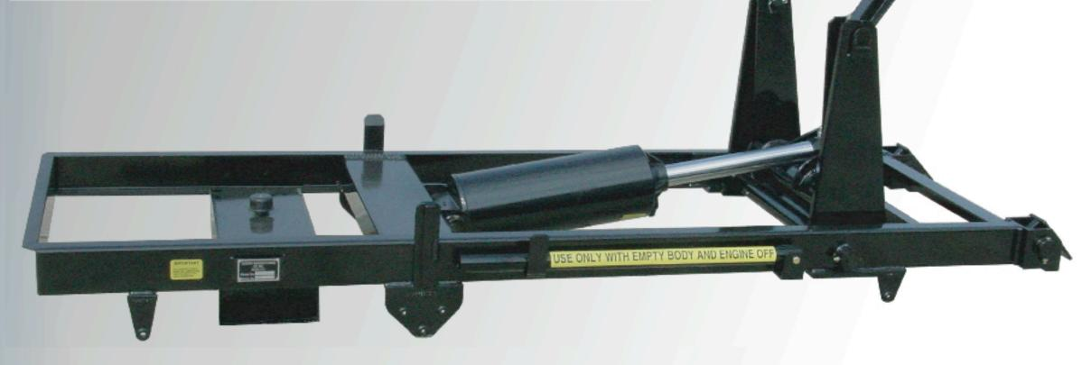
Champion built cylinders and hoists are designed to be double acting (power up and down). Our hoists are easy to install with as little truck and body modification as possible. To further ease the installation process, Champion hoists mount to the body and truck chassis using heavy duty grade 8 bolts with little or no welding needed.
